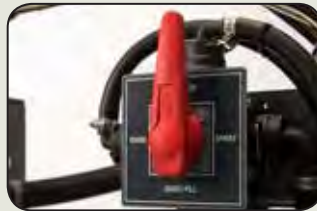
Plumbing control valve
