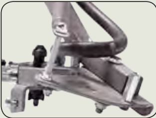
Boom folding and breakaway mechanism on 13' and 20' models
