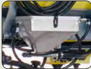
Chemical eduction system
